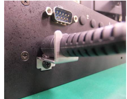
Step3: Lock with M3 screw
