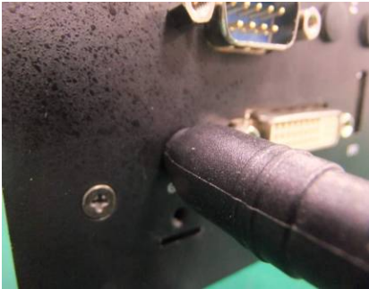
Step1: Install the DC plug
