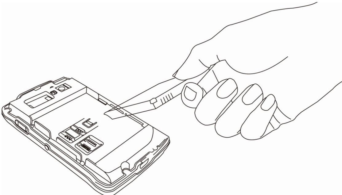
4. Insert the SIM card (with its gold contacts facing down and cut-off corner facing out) all the way into the SIM card slot.
