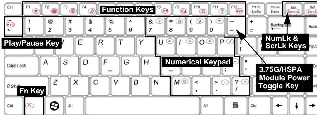
Figure 1 - 6 - Keyboard - Model A
