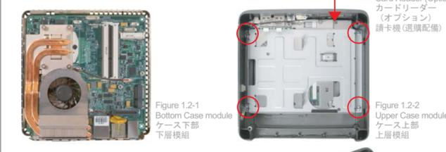
1.3 Remove four screws of the supporter. Take the riser card / card reader module from the little bag.
