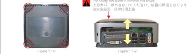
1.2 Distribute the Bare bone into two modules. \* Bottom Case module. \* Upper Case module.
