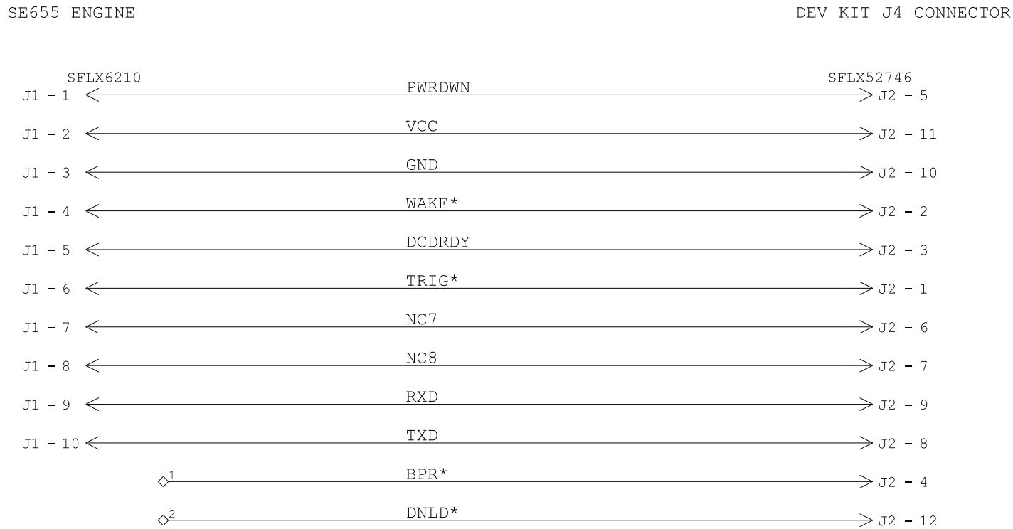
NOTE: BRING TEST POINTS 0.5 IN TO J1 Figure 2-12 Flex Strip 15-141354-xx, Schematic
