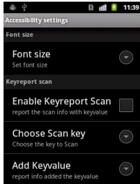
2. Click “Choose Scan key”, see as the picture. Choose “none”,then the orange key do only as enter key. Choose the “Change enter to scan”, then the orange key becomes a scan key and only do as scan key in demo. And the others like F1,F2 and F3 do only focus on the Focus Scanning while unrelated to specific demo.
